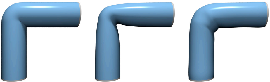
Figure 4: A cylinder is bent by explicitly deforming its base surface, which is a cylinder of half the radius. Normal displacements immediately lead to local self-intersections (left), whereas our new technique effectively avoids them (center). Compared to the non-linear displacement volumes [2] (right) our linear method does not (try to) preserve volume.
