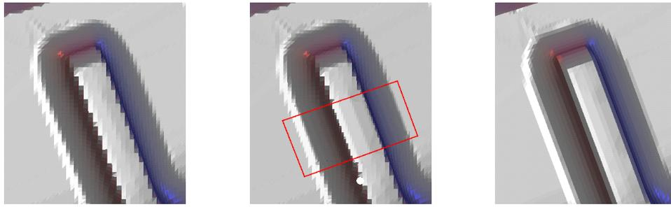
Figure 1: At sharp feature lines, any sampling algorithm tends to generate alias artifacts (left) which cannot be removed by refining the sampling density (center). However, aligning the sampling grid to the feature improves the visual quality.
